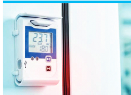
The data logger can be fixed to deep-freezers magnetically and configured or read via a USB interface
